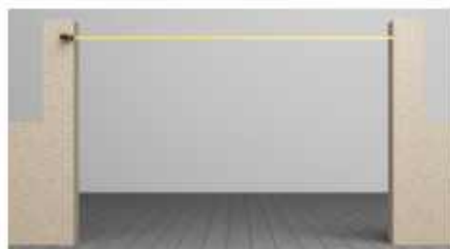
5 Mesurer en haut. Retenir la plus petite mesure: Measure the distance between pillars at the top. Consider the smallest distance: bottom, middle, top.
